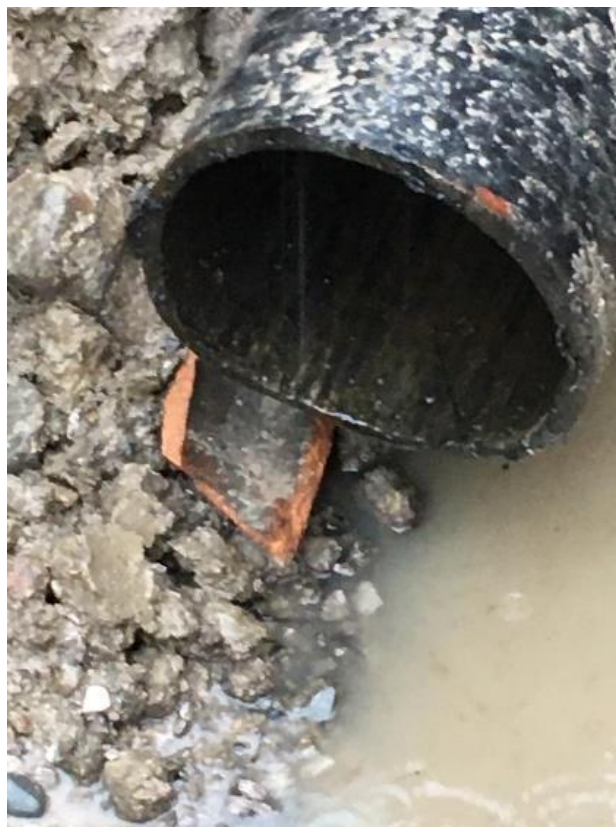
Fig 3 Original pipe, in poor condition as taken out of service
