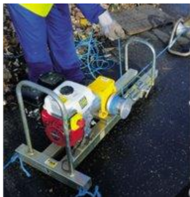
Fig 1: Aqualiner winch to pull liner
