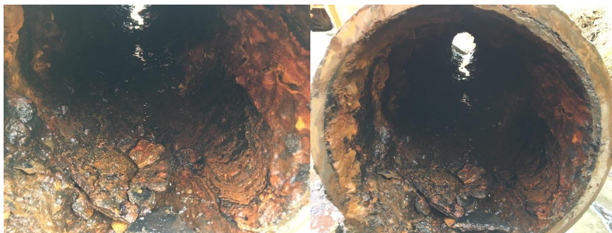
Fig 4: photographs of the inside of the cast iron pipe showing severe corrosion
